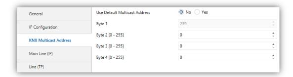
Figure 18 KNX multicast address configuration tab.
