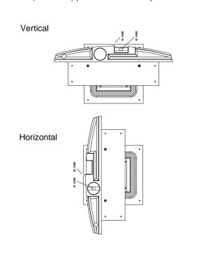
**3** Fix the accessory to the dry-wall frames with suitable screws (not included). Once fixed, the *auxiliary mounting part* can be removed by taking the two screws off.
