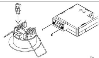
Make a circular hole with a diameter equal to 40 mm.
