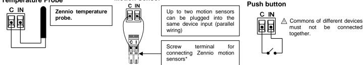
\* In case of using ZN1IO-DETEC-P sensor, its micro switch number 2 must be in **Type B position**.
