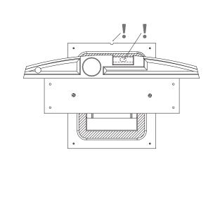
**3** Fix the accessory to the dry-wall frames with suitable screws (not included). Once fixed, the *auxiliary mounting part* can be removed by taking the two screws off.
