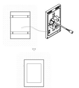
The device can be removed by pressing the device on the bottom area to make it tilt [1]. Afterwards, it can be removed [2].
