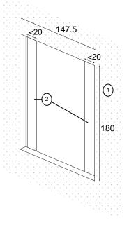
Place the accessory into the hole and adjust the exact position with the help of a level.
