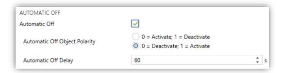
Figure 14. A/C Gateway. Configuration. Automatic off.
