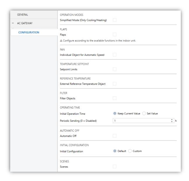
Figure 6. A/C Gateway Configuration
