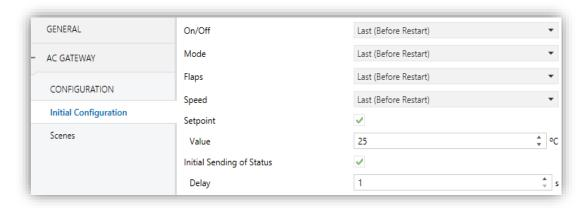
Figure 17. A/C Gateway. Initial Configuration.
