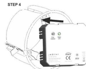
**Installation note:** Make sure that no wires are pinched or squeezed when placing the device into the hollow-wall box.
