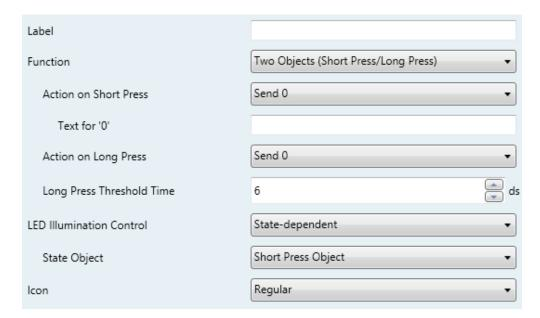
Figure 41 Individual Button – Two Objects (short press / long press).
