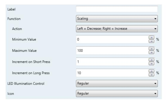
Figure 26 Pair Buttons – Scaling.
