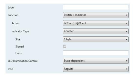
Figure 22 Pair buttons – Switch + Indicator.
