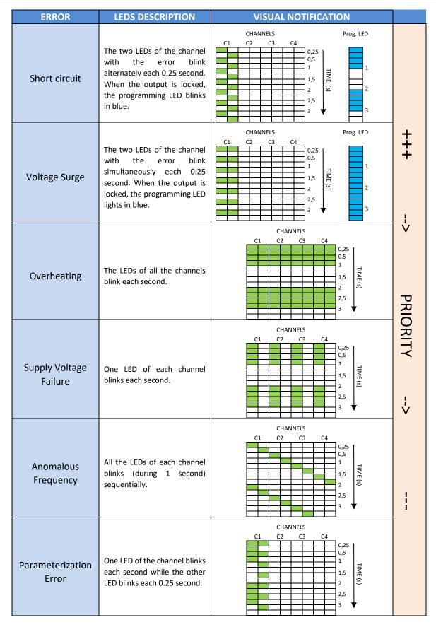
Table 2 Error Notification through the on-board LEDs.
