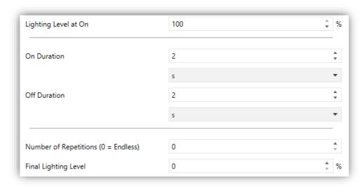
Figure 14 Flashing.
