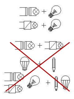
Figure 2. Combining Load Types.
