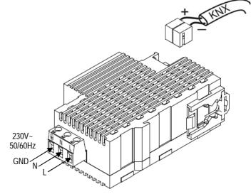
Figure 2: ZPS160MPA installation and connection
