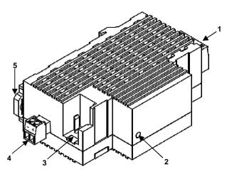
Figure 1: ZPS160MPA power supply
