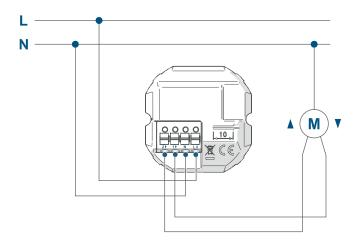
A neutral conductor is required for installation
