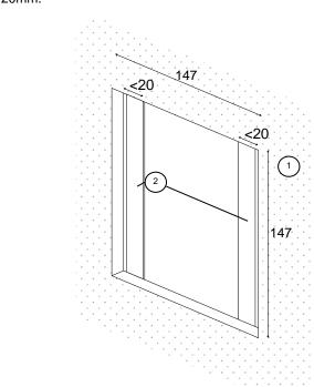
2 Place the accessory into the hole and adjust the exact horizontal (or vertical) position with the help of a level.
