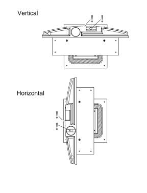
**3** Fix the accessory to the dry-wall frames with suitable screws (not included). Once fixed, the *auxiliary mounting part* can be removed by taking the two screws off.
