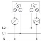
Figure 2: Wiring example (from left to right): three-speed fan, load and open/close valve, load and open/close valve to different phases.
