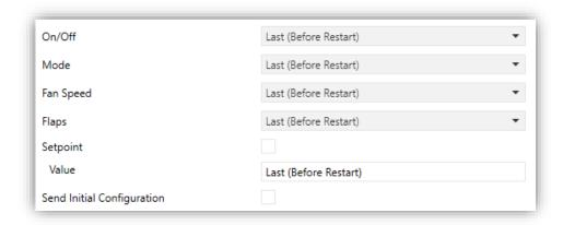
Figure 18. A/C Gateway. Initial configuration.
