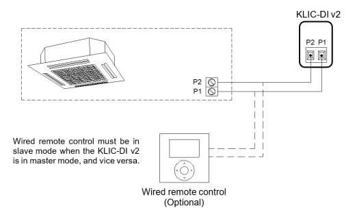
Figure 2. Connecting KLIC-DI v2 to the P1/P2 bus.
