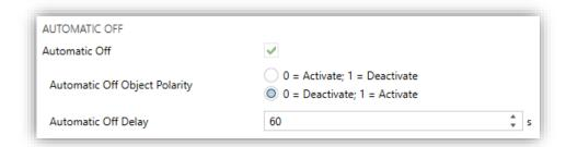
Figure 14. A/C Gateway. Configuration. Automatic off.
