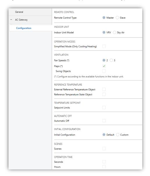
Figure 6. A/C Gateway. Configuration.
