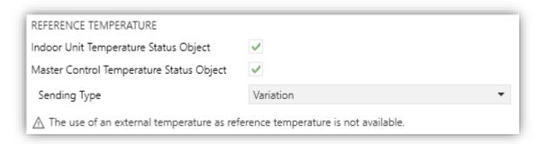
Figure 12. A/C Gateway. Configuration. Reference temperature (slave control).
