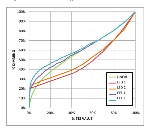
Figure 11 Dimming Patterns for LED and CFL loads.
