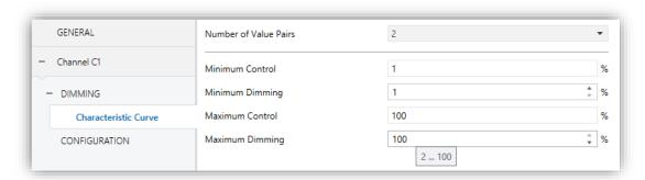
Figure 12 Characteristic Curve.
