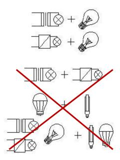
Figure 2. Combining Load Types.
