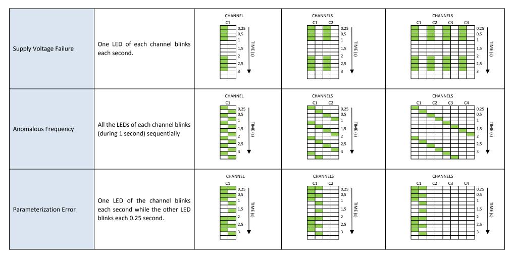
Table 2 Error Notification through the on-board LEDs.
