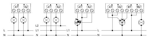
⚠ In order to ensure the expected status of the relays, please check that the device is connected to the KNX bus before energizing the power circuit.
